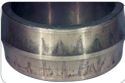
Water contamination of bearings can degrade lubrication causing wear and corrosion damage
